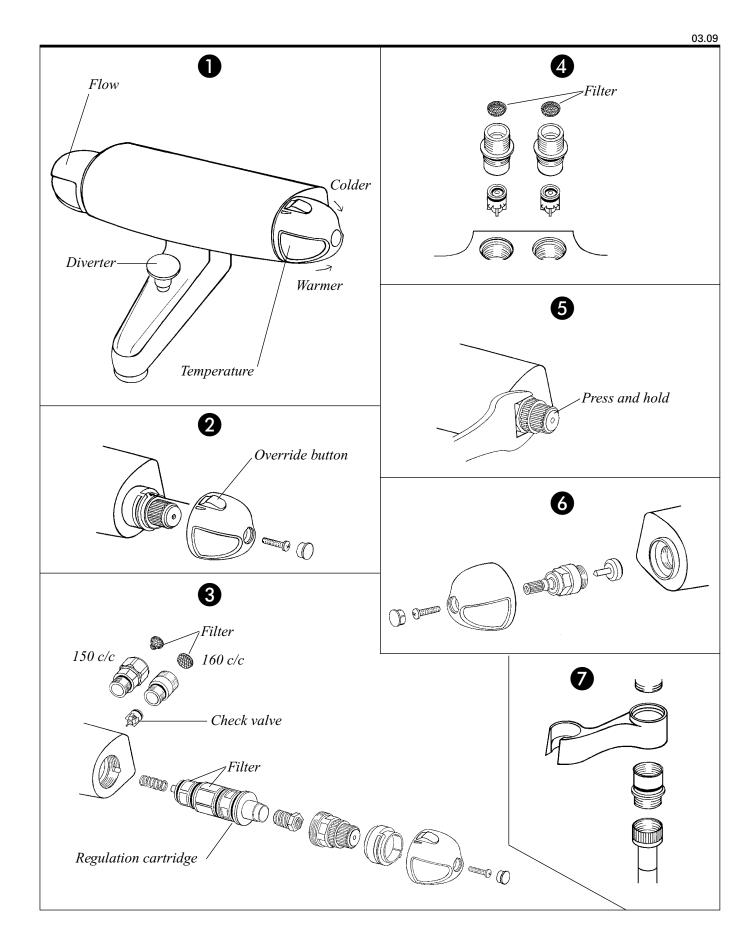
Always close the main supply valve before maintenance (service). (Except for when calibration of temperature is performed).
